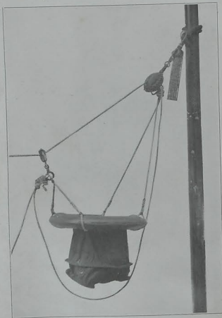
Breeches Buoy fitted with metal snatch block for whip apparatus.
